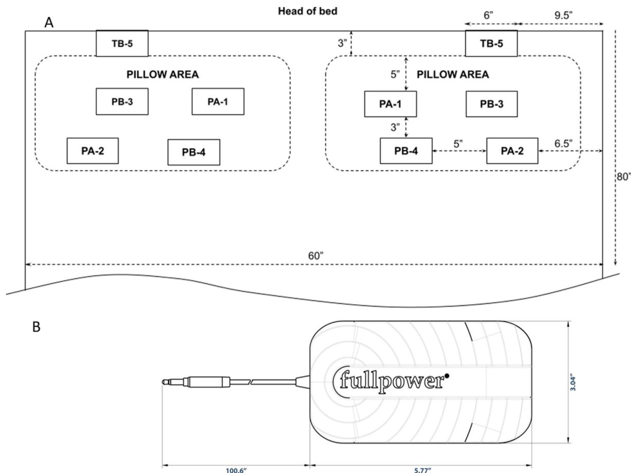
**Fig. 1.** One Sleeptracker-AI Monitor setup consists of two Sleeptracker-AI Monitor sensors placed between the mattress and foundation, each connected to one Sleeptracker-AI Monitor processing unit.
